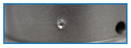
The CM Round punches are perfect for material deformation. The results are clear and may be used as an acceptance mark.
