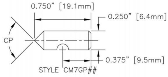
The model 78 is used in combination with the CM7 Prick Punch to provide disruption of threads as a locking application.
