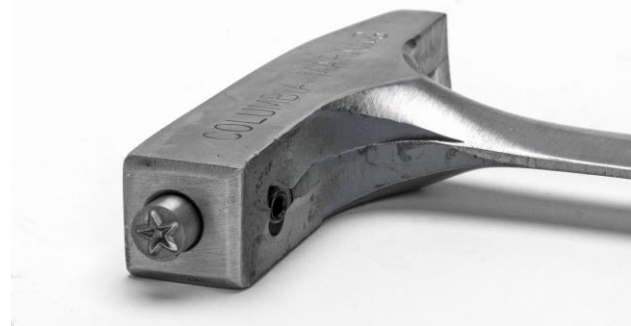
impact marker Model 88 and 288 "OB" rod retained with a set screw. They are also used in the #8 Inspectors hammer.
