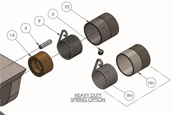
CMT. offers a **HEAVY-DUTY** upgrade for the return spring. The return spring is a normal wearable component, and for large and heavy tooling the normal spring will require more changes. CMT recommends upgrading to the heavy-duty spring and housing for applications requiring extended tool life.
