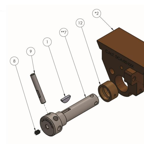
XXX – While most of the details of the DCA series are interchangeable the SHAFT and the FRAME are unique to the cataog number. Replace as follows
