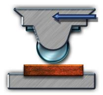
Example showing dovetail roll carriage with solid concave roll die marking along the OD of a round part.
