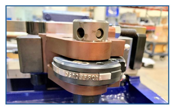
The roll type holder in combination with the dovetail roll carriage minimizes changeover times and reduces tooling costs.
