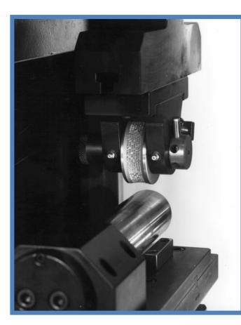
A key element in the roll marking process of marking on flat parts is the roll carriage.
