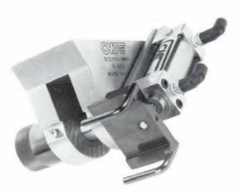
Columbia's combination roll carriage and automatic actuator advances roll style numbering heads to the next consecutive number after every cycle of the marking machine. Then the carriage rotates the head through the roll marking process. Completely pneumatically operated, the actuator is furnished with a cylinder, roll carriage, and valve pack. Designed for today's high production, automatic lines, it features oversize bearings, quick disconnect air fittings, and hardened wear surfaces.
