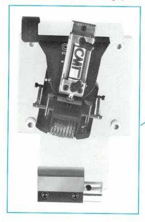
Due to the rolling action of the convex head, only part of the marking legend contacts the surface at any one time. Pressures for roll marking vary in terms of the number of characters in contact with the surface, character size, material, and the marking radius.
