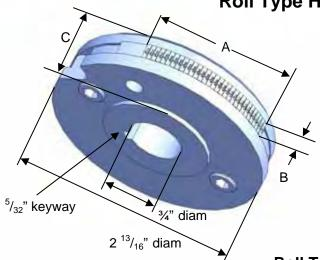
COLUMBIA roll type holders, developed to efficiently mark both flat and contoured surfaces, are designed to hold individual step style wedge type or combinations of wedge type, logo-type, and segment dies. The step in the cover plate retains the type in the holder while a take-up plate, provided with each holder, holds the type in perfect alignment.
