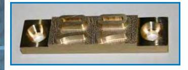
**Extra Deep Engraving:** Required when material is removed from a part after marking or for an abnormally deep mark. Branding dies are engraved extra deep with a flat face so the background of the hot die will not touch the material.
